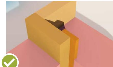
A two stud corner with a small nailing strip or drywall clips is a great alternative.
