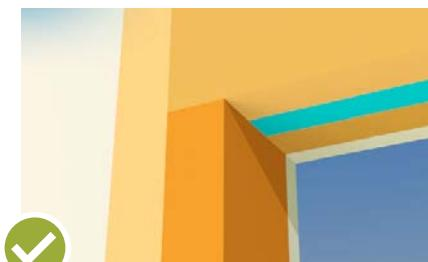
Header insulation will replace the often used OSB filler.
