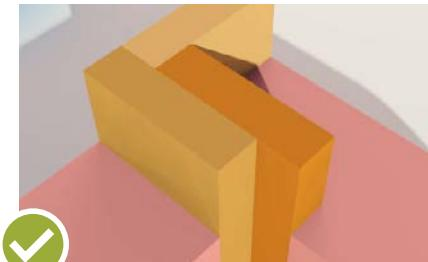
This is a three stud, or "California" corner which allows for max insulation coverage.
